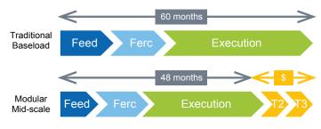
Modularization facilitates faster, cost effective construction. Trains can be brought on-line independently for earlier revenue.
