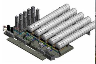
Chart designed, built, installed and commissioned the complete cryogenic section for the small-scale import terminal to establish the Lithuanian port of Klaipeda as an LNG distribution hub for the Baltic region. The Chart solution enables LNG offloaded at the terminal to be used for marine bunkering, loaded into road tankers for small-scale distribution and re-gasified for pipeline transmission.
