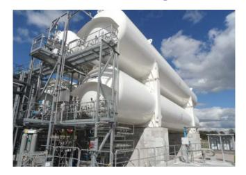
A 4-pack stack of 300 m<sup>3</sup> horizontal tanks minimizes footprint for the storage of nitrogen and oxygen.
